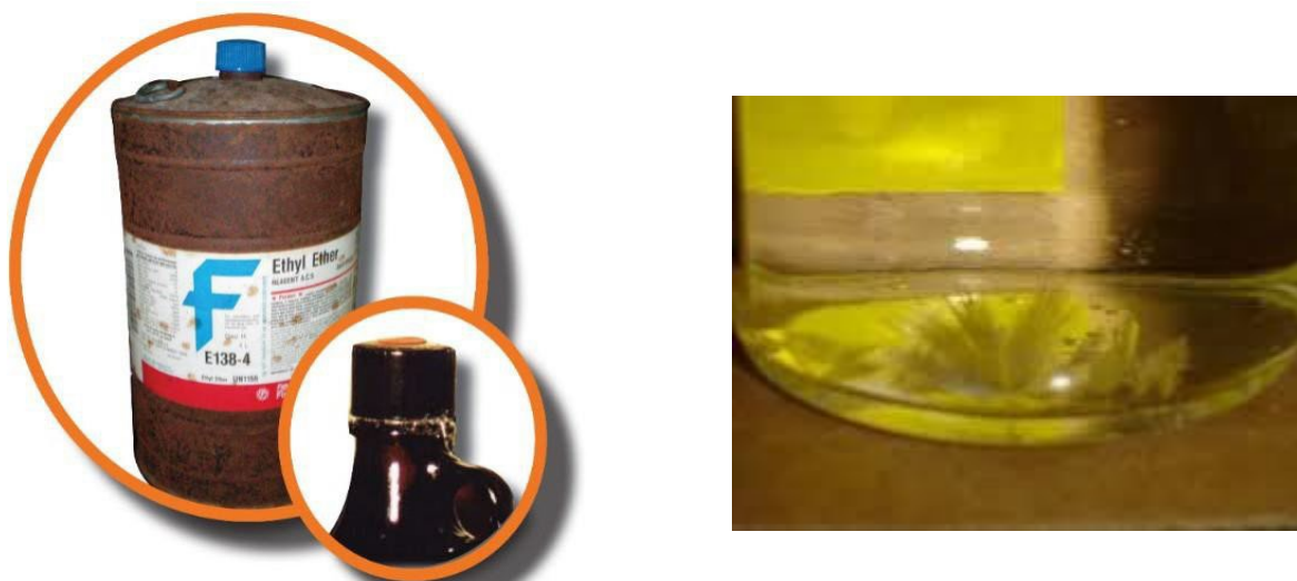
Figure 1. Examples of chemical containers showing signs of crystal formation
