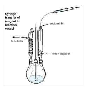
Fig. 2C Syringe transfer of reagent to reaction vessel
