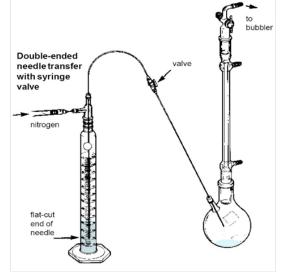
Fig. 3C. Double-ended needle transfer with syringe valve
