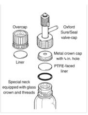
Fig. 1A Sure/Seal components
