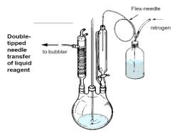
Fig. 3A. Double-tipped needle transfer of liquid reagent
