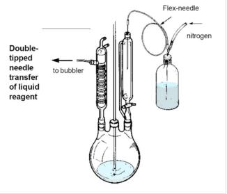
Fig. 2 Double-tipped needle transfer of liquid reagent
