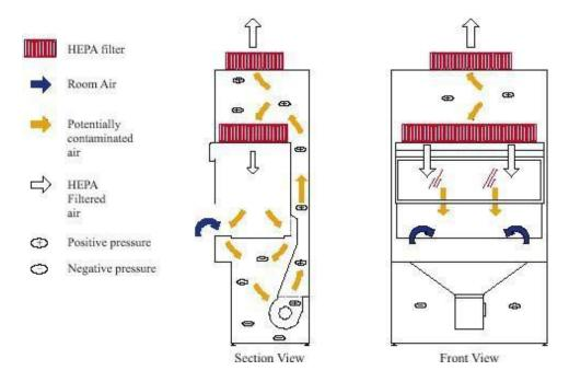
**Class II, type A2 or A/B3:** this does not have to be vented, which makes it suitable for use in laboratory rooms which cannot be ducted. 30% of the air is exhausted from the cabinet while 70% is recirculated. This cabinet may be used with etiologic agents treated with minute quantities of toxic chemicals and trace quantities of radionuclides that will not interfere with work if recirculated in the downflow air when ducted.
