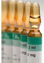
Ampoules used to store biohazardous material in liquid nitrogen have exploded causing eye injuries.
