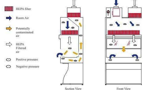
within the Class III cabinet are conducted through attached rubber gloves. When in use, the Class III cabinet is maintained through negative air pressure of at least 0.5 inches water gauge. Supply air is drawn into the cabinet through HEPA filters. The cabinet exhaust air is filtered by two HEPA filters, installed in series, before discharge outside of the facility. The exhaust fan for the Class III cabinet is generally separate from the exhaust fans of the facility's ventilation system.
