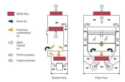
**Class II, type B2**: this cabinet must be totally exhausted, with 100% of the air exhausted through a dedicated duct. This cabinet may be used with etiologic agents treated with toxic chemicals and radionuclides required as an adjunct to microbiological studies.
