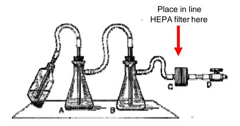
If a glass flask is used at floor level, place it in a plastic container that is large enough to contain any spilled liquid to prevent breakage by accidental kicking. Do not use absorbable material, such as cardboard or Styrofoam, as a secondary container. In BSL2 or higher laboratories, the use of Nalgene flasks is recommended to reduce the risk of breakage.
