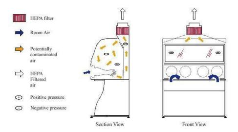
**Class II** biological safety cabinets are designed to protect the worker, the general public and the product. The airflow velocity at the face of the work opening is at least 75 linear feet per minute (lfpm). Both the supply and the exhaust air are HEPA- filtered. This is the most common class of biological safety cabinets found on campus.
